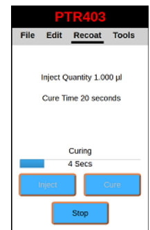
Click to Enlarge Screenshot of VYT300C Controller When Used with PTR403 Recoater
